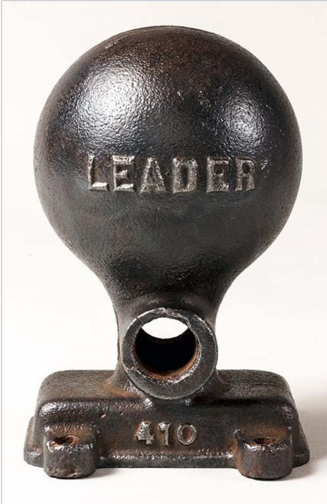
Fig. 1 (left): Front view. The back view is identical to this front view, except there is no embossing. The passageway above "410" goes through the casting to the back. Its openings are 1 3/16" in diameter and each end is internally threaded. PHOTO: © 2018 Richard W. Black
