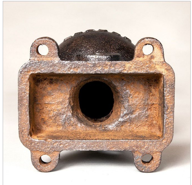
Fig. 2 (below): Bottom view. The hole in each of the four "ears" is \frac{3}{8} " in diameter and is not threaded. The hole in the center is also not threaded and freely connects to both the passageway and the globe seen in figure 1.
